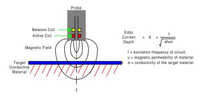
The test system places an exciting coil that generates a high frequency magnetic field close to (but not touching) the target specimen to create the eddy currents. These induced currents produce a secondary magnetic field. Measuring the resulting field composed of the primary and fields, secondary the sensor receives the target specimen
